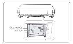
**4** Find the PCB wire, and connect the wire to the Sub PCB as seen in the picture.
